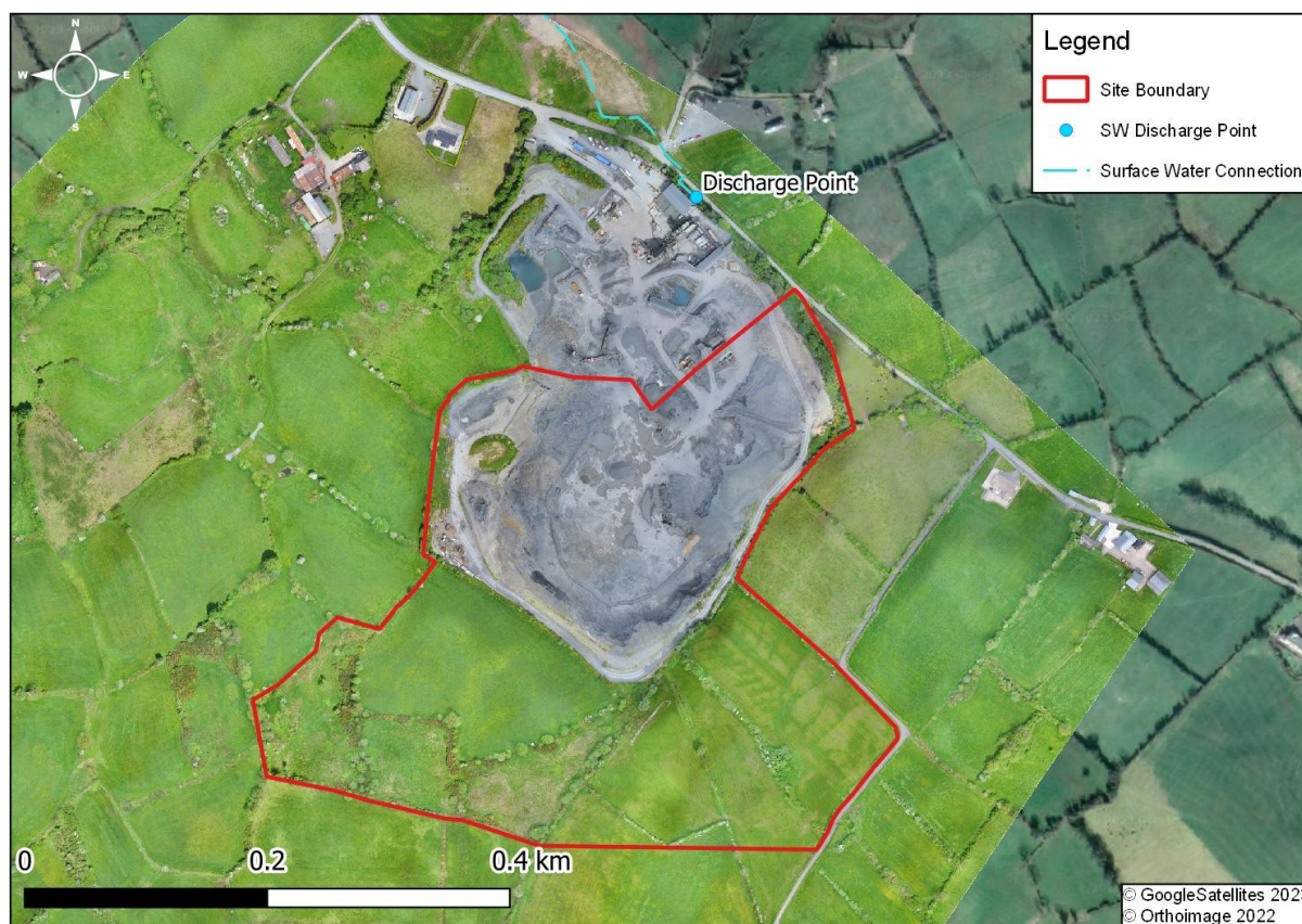
Figure 3-2: Discharge Licence Drainage
